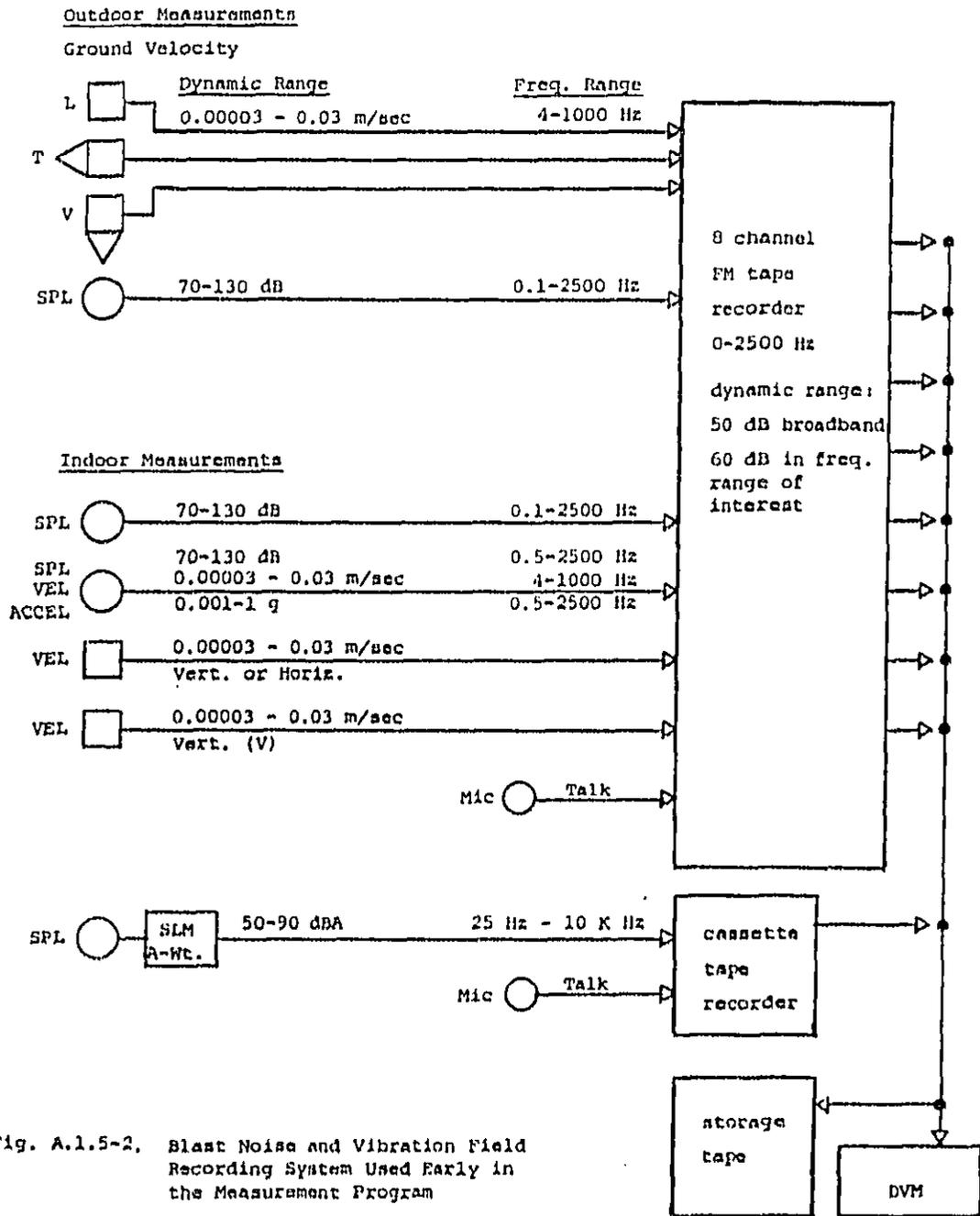
Fig. A.1.5-2. Blast Noise and Vibration Field Recording System Used Early in the Measurement Program
