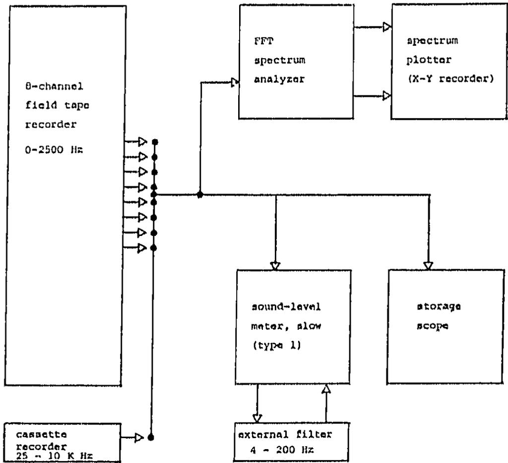
Fig. A.3.3-1. Data Analysis System for Determining Blast Noise and Vibration Spectrum, Peak and Various Sound-Level Meter Descriptors
