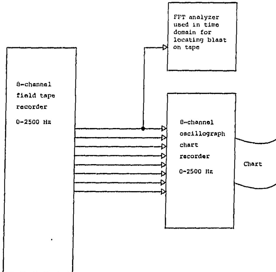
Fig. A.3.2-1. Simultaneous Time History Analysis of Eight Noise and Vibration Signals Recorded During a Single Blast Event
