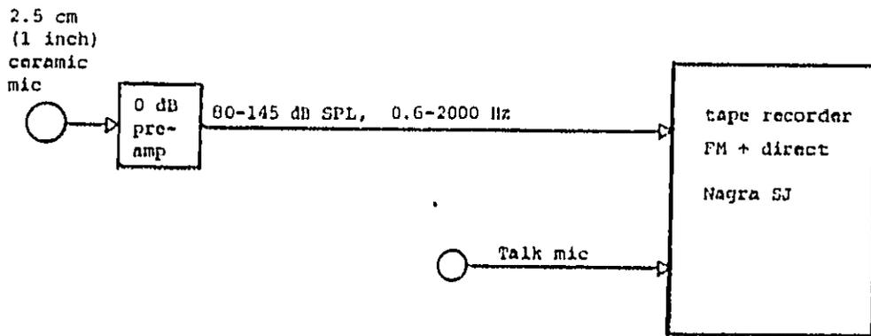
Fig. A.2.2-1. Portable Air Blast Recording System Used by Illinois EPA Personnel for the 1975 IEQ and 1976 EPA Quarry Blast Noise Study
