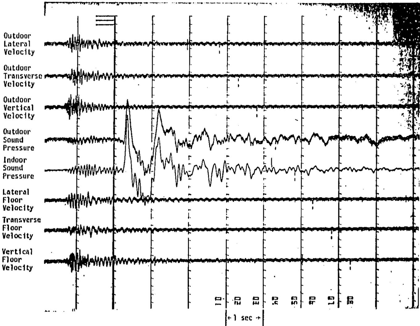
Fig. B-6. Oscillograph Record of Blast No. 6
