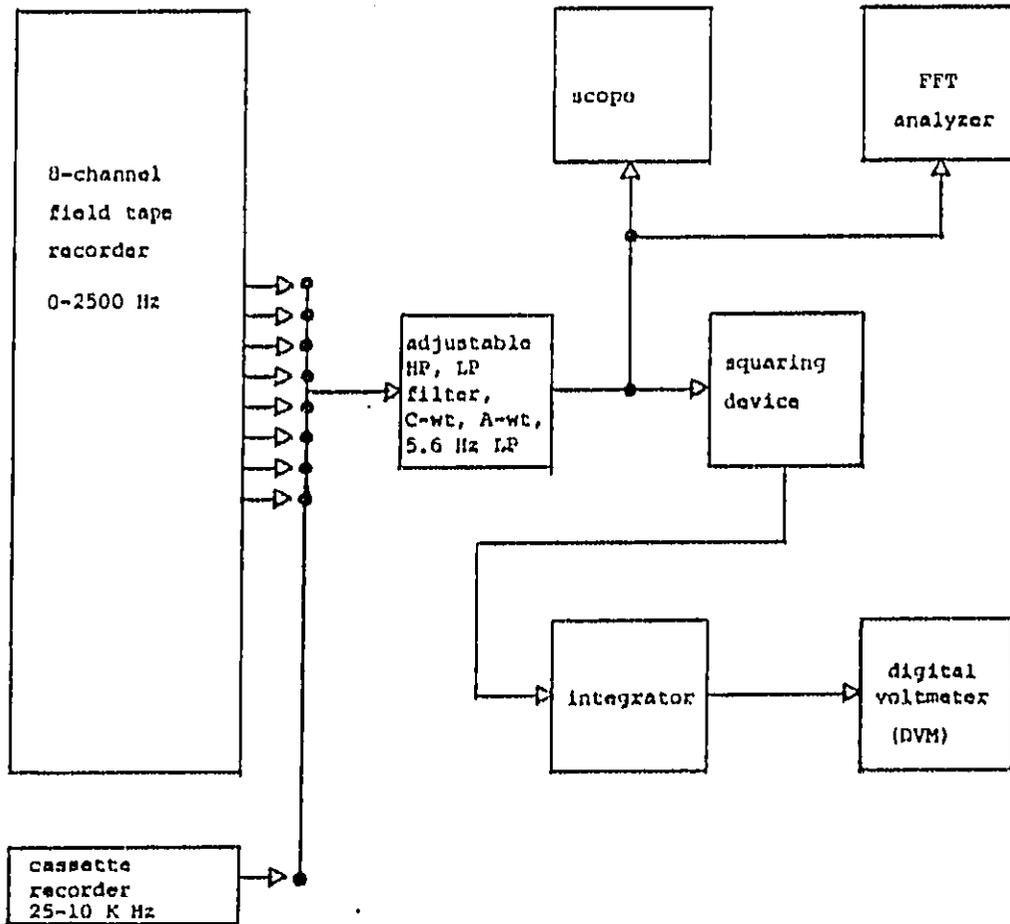
Fig. A.3.4-1. Data Analysis System for Determining Blast Noise and Vibration Energy, SEL and VEL.
