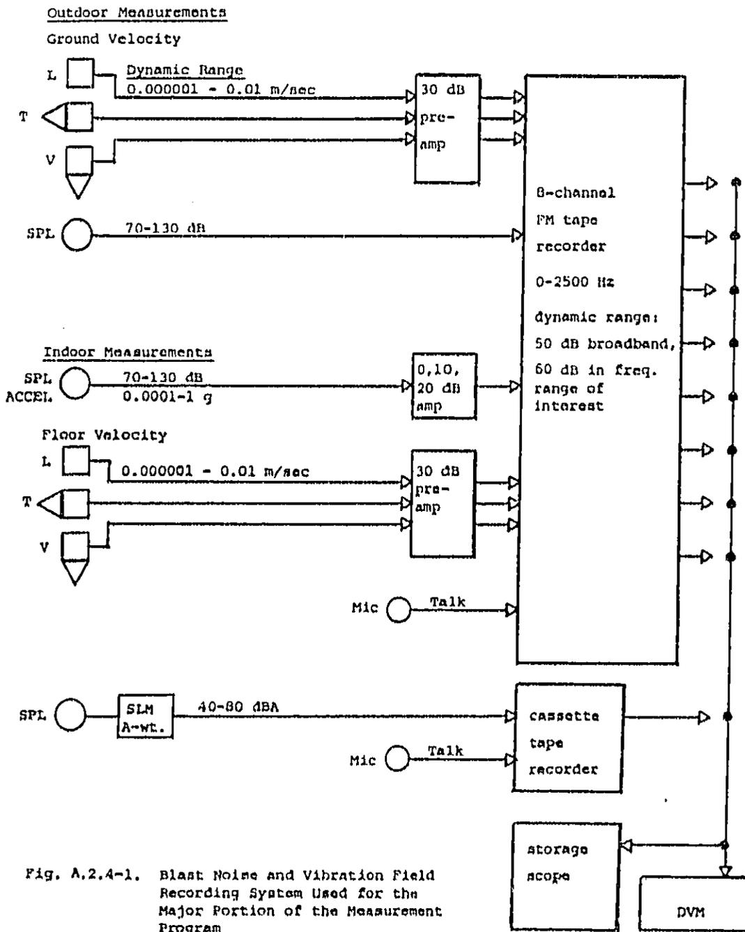
Fig. A.2.4-1. Blast Noise and Vibration Field Recording System Used for the Major Portion of the Measurement Program
