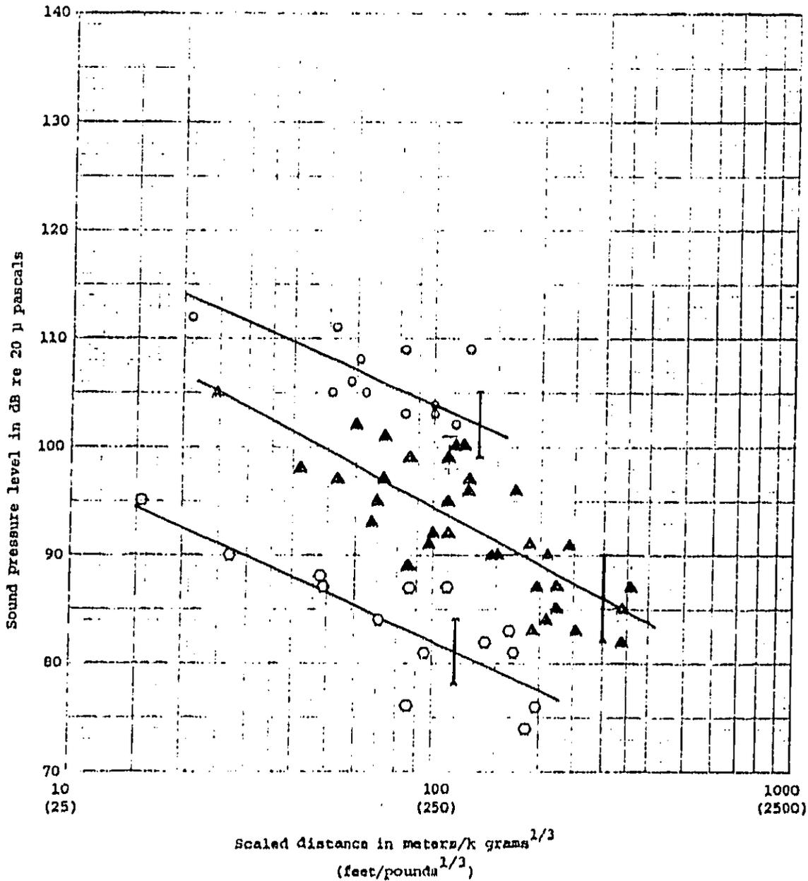
Fig. 3.7-4. Sound Levels versus Scaled Distance
